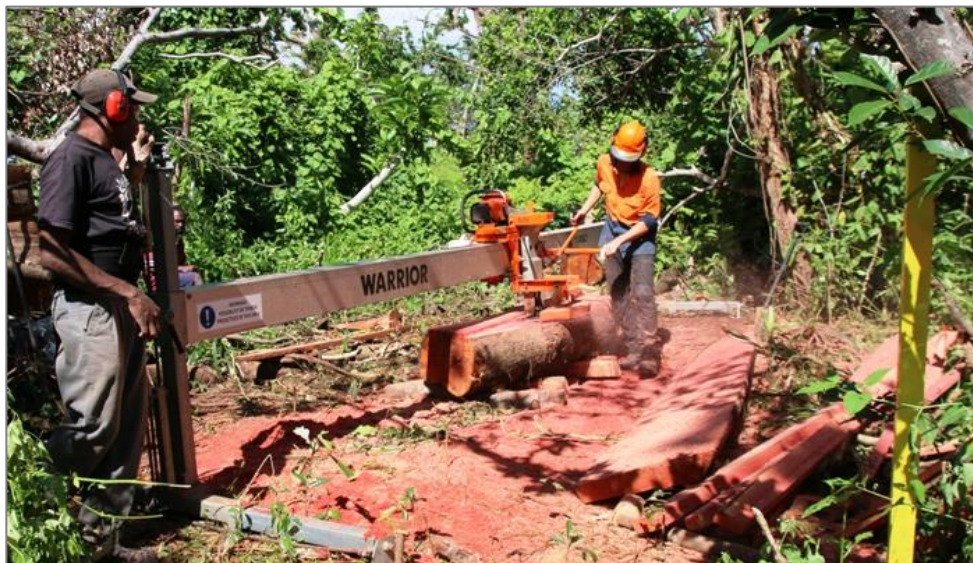
Figure 9 – Example of portable sawmill in Tanna, Vanuatu / TC Pam recovery (photo credit: Faisal Ridwan)
