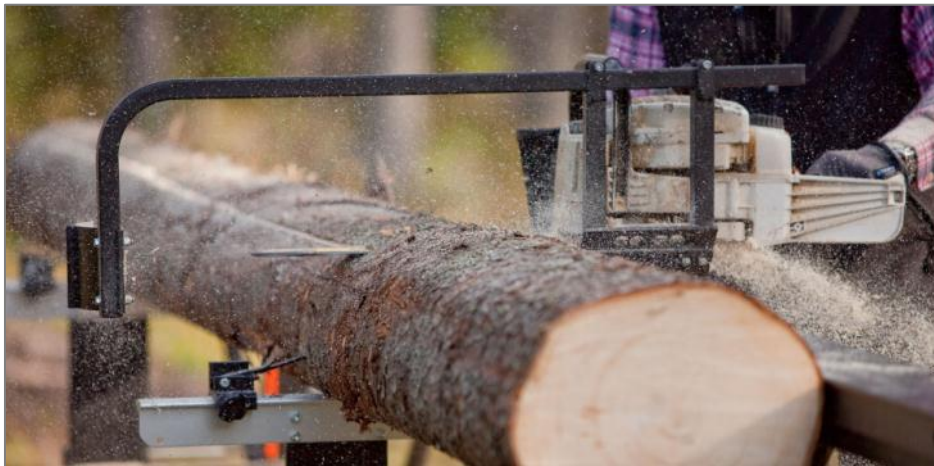
Figure 8 – Example of portable guided chainsaw mill (source: http://www.logosol.us/sawmills/m8/ )
